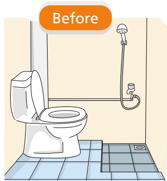
Toilet flooring that is not level due to step-down shower area.
