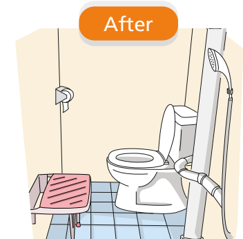
Installation of foldable shower seat against the wall.
