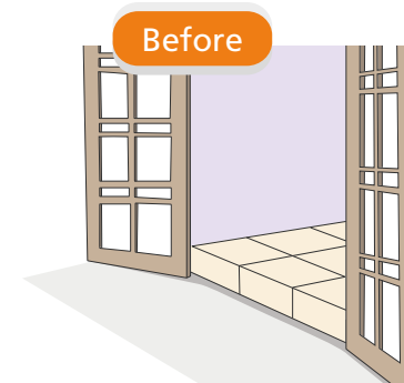
Presence of kerb at door entrance
