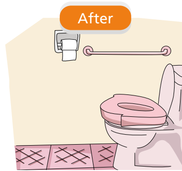
A sitting toilet with an additional toilet raiser, installation of grab bar and anti-slip floor treatment
