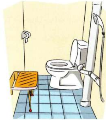
After: Installation of foldable shower seat against the wall.
