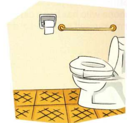
After: A sitting toilet with an additional toilet raiser, installation of grab bar and anti-slip floor treatment.
