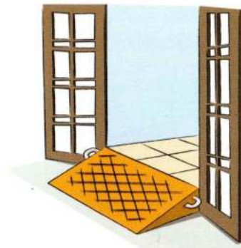
After: Installation of removable wooden ramp with non-skid covering.
